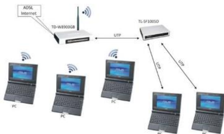
Wi-Fi ADSL modem - TP-LINK: TD-W8910GB - ADSL2+ modem, AP , Router (Annex B)
